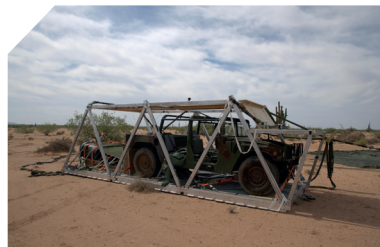
Fig 3: Air bag landing, de-rig <10 mins
